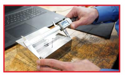
All tool steel is carefully inspected to insure material quality and size accuracy.
