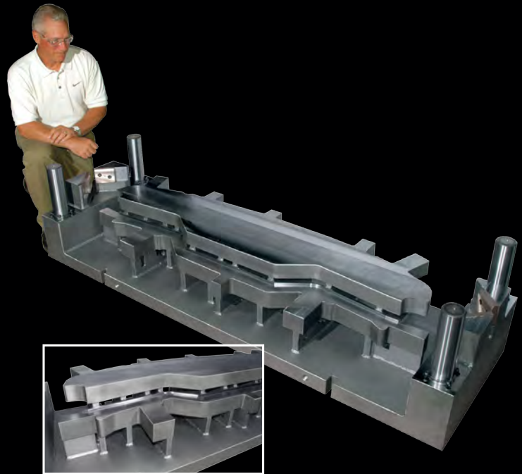
Fabricated trim block with "V" Wear Plate system
