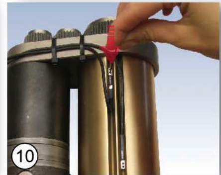
10 Use the core puller control system to move the core into its final limit position. Adjust the magnetic field sensor causing the LED to light up. The hydraulic pressure should be 20-25 bar above the run-in pressure, ie. about 60-65 bar.
